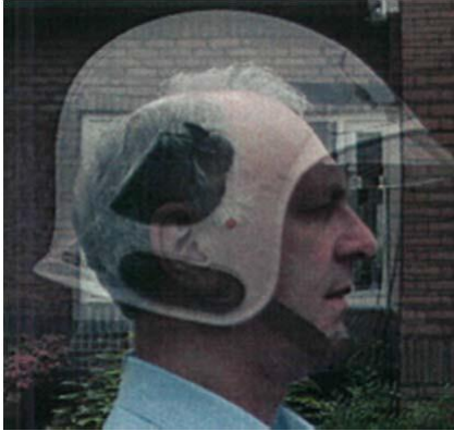
Fig. 9. Superimposed images of a photo of a head and head/helmet combination to provide insight in fit.
